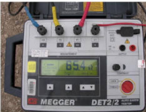
*Photo showing final reading of the Poly-Ground installed pole. Reading is 65.4 ohms.*
